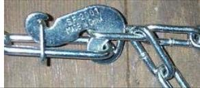
Step 3. Move tire until fasteners are axle high.
