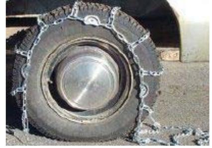
Step 2. Lay chain over tire, cross chain hooks up and fastener on outside of tire. Tuck first cross chain under tire.
